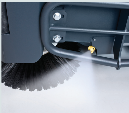
The Nilfisk DustGuard™ system reduces up to 85% of airborne dust generated by side brush when sweeping
